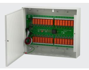
The 32 way relay panel accepts relay data from the combi control unit. It must have a unique address between 128 and 255. This can be selected using the SW1 binary address switch (see example). Ensure that its address does not conflict with another CAN bus device.
